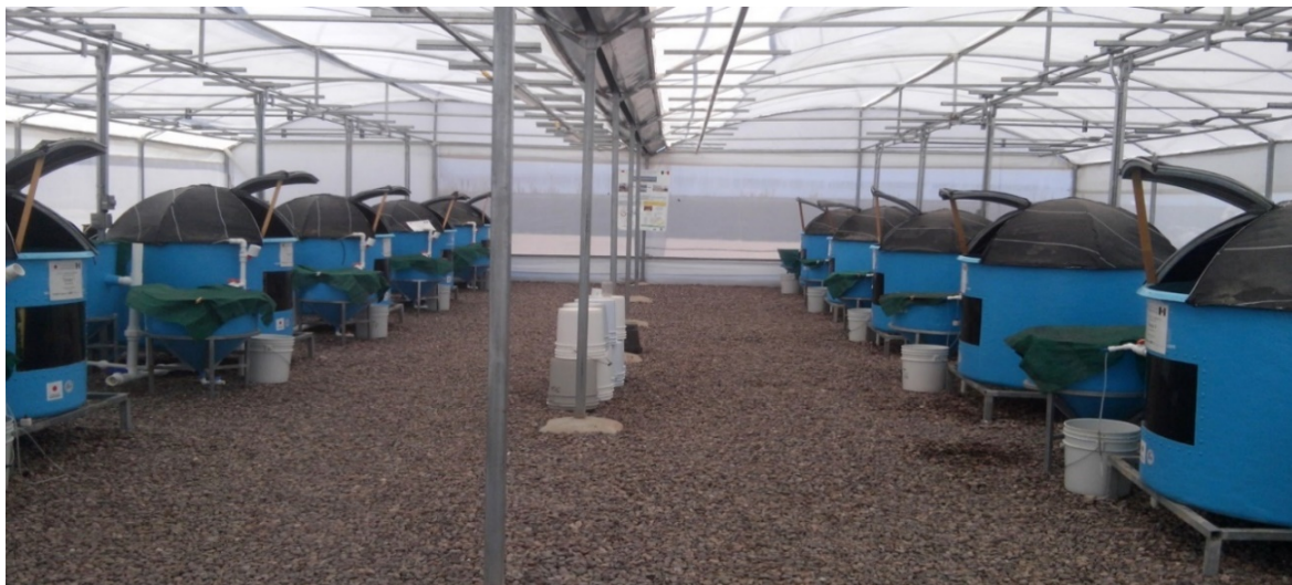
Figure 12. Recirculating Aquaculture System conformed by 12 individual units with recirculation. The tanks were covered with a black mesh dome (60% light retention). The tanks, settlers, bionitrifiers and mineralizers were manufactured with fiberglass, coated with high quality epoxy paint blue color.
